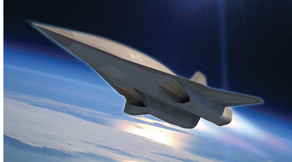
High Speed ISR/Strike Aircraft concept, Mach 6 TBCC. Source: Lockheed Martin
