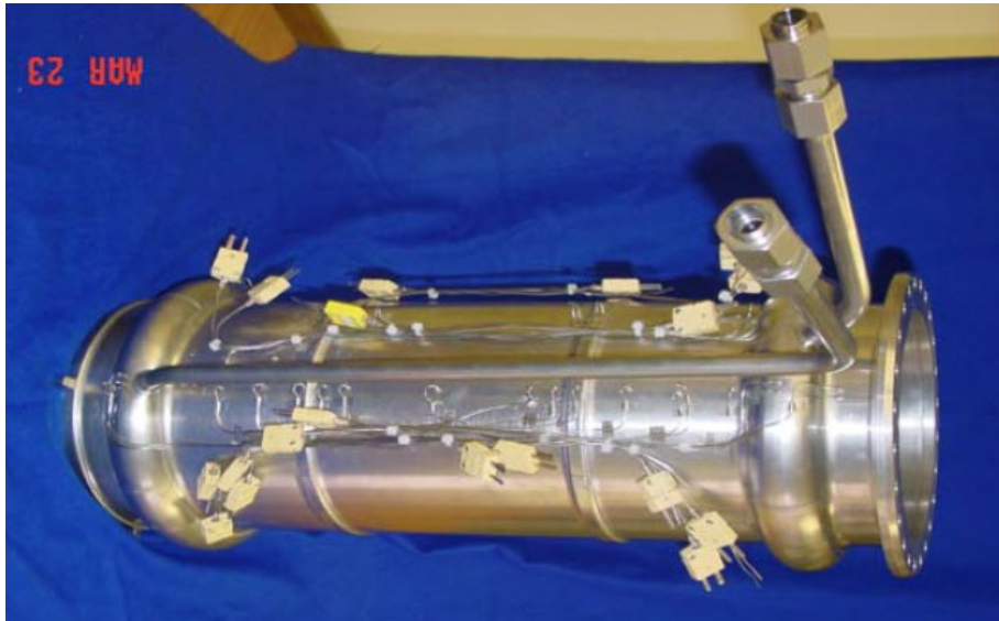
Fuel-cooled, flight-weight, circular scramjet combustor by Northrop Grumman (ATK GASL), Bakos (2008)
