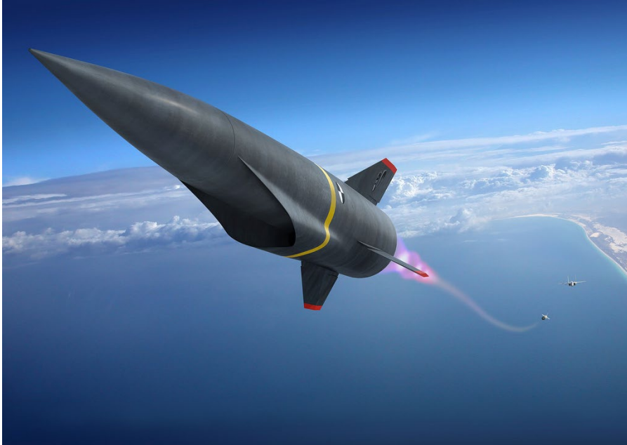
High Speed Strike Weapon concept, Mach 6 missile demonstrator. Source: Lockheed Martin
